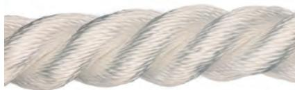
The softness and high tenacity characteristics of polyester are complemented in this rope by a balanced twist construction that enhances its excellent resistance to heat and abrasion, creating a durable, high tenacity rope with low elongation and excellent durability.
