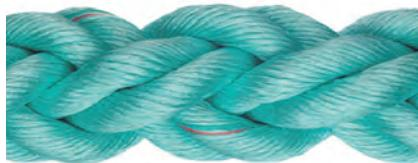
Polysteel is an extremely strong, high tenacity bi-polymer composite fiber extruded in a custom extrusion process. Its gripping ability is enhanced by the diffuse outer surface, which protects the inner fibers against abrasion.
